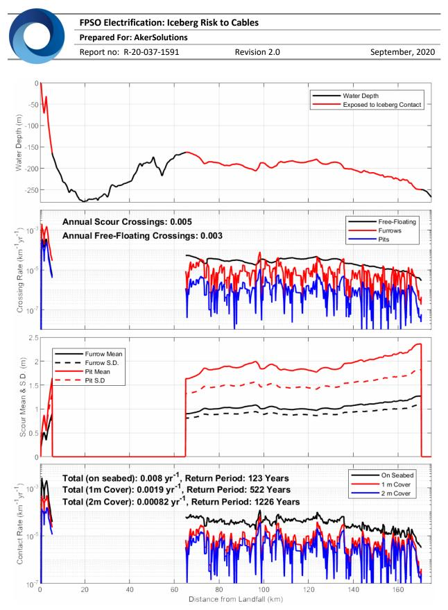
Figure 21. West Orphan Basin cable risk analysis (Conception Bay landfall): portions of route exposed to icebergs, iceberg crossing rates over the cable, furrow and pit depth parameters, and contact rates
