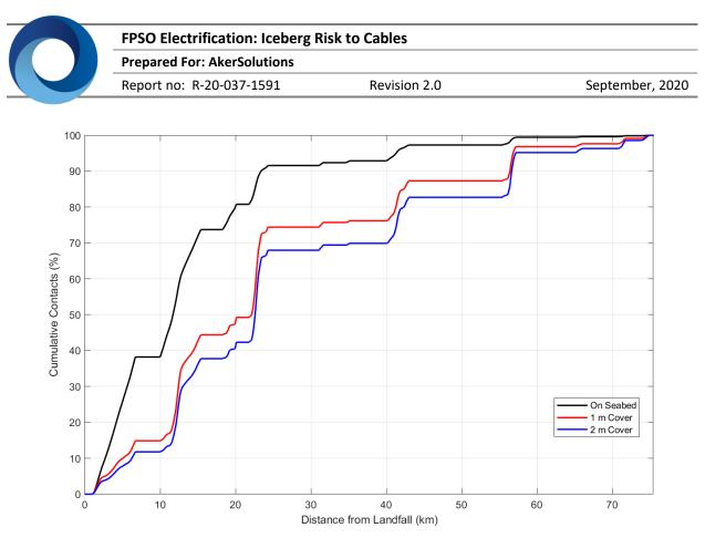
Figure 17. Cumulative contact rate along route for cable on seabed and trenched with 1 and 2 m cover
