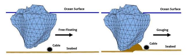
Figure 2. Iceberg interaction with a cable on the seabed
