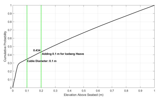
Figure 12. Proportion of free-floating iceberg keels within 1 m of seabed capable of contacting cable
