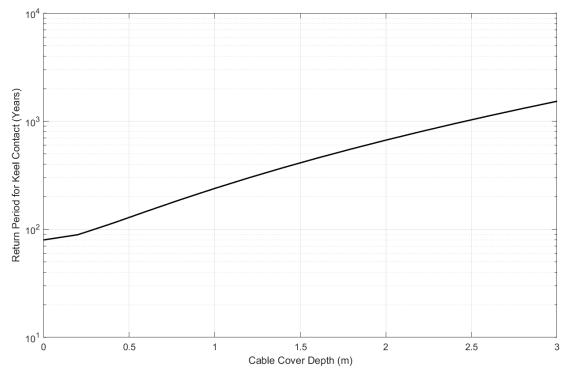
Figure 18. Mean return periods for cable contact as a function of cover depth
