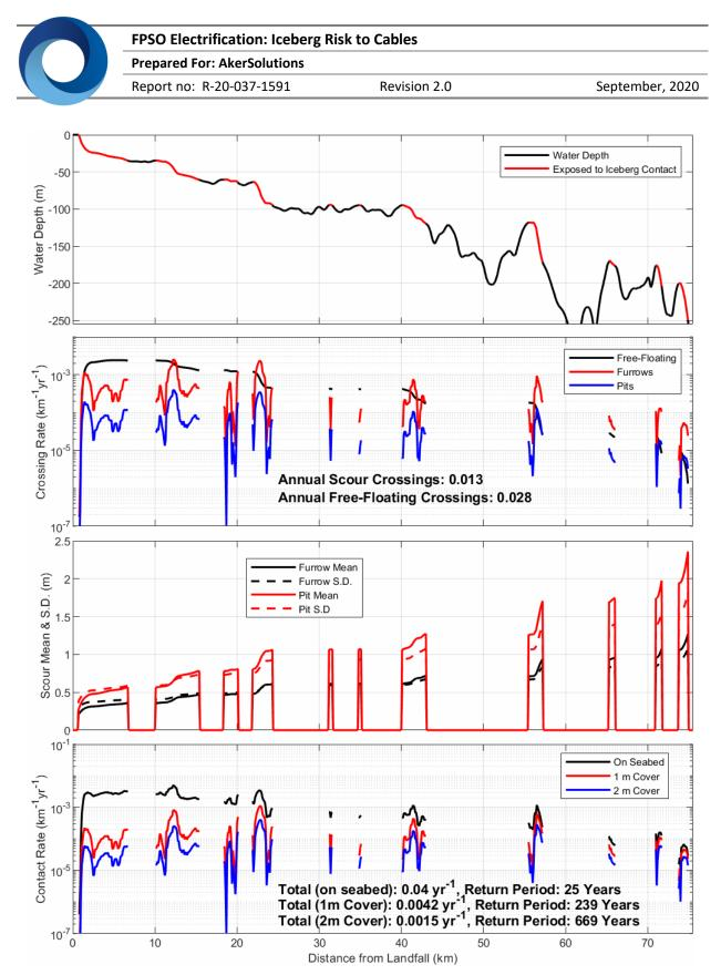
Figure 16. Labrador South cable risk analysis: portions of route exposed to icebergs, iceberg crossing rates over the cable, furrow and pit depth parameters, and contact rates
