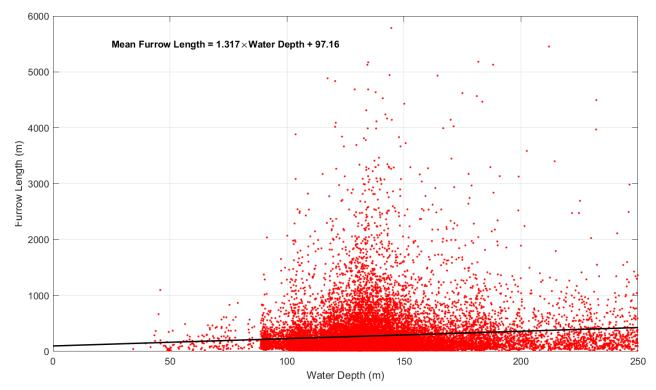
Figure 7. Mean furrow length as a function of water depth, Makkovik Bank region
