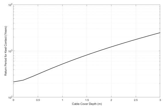
Figure 23. Mean return periods for cable contact as a function of cover depth
