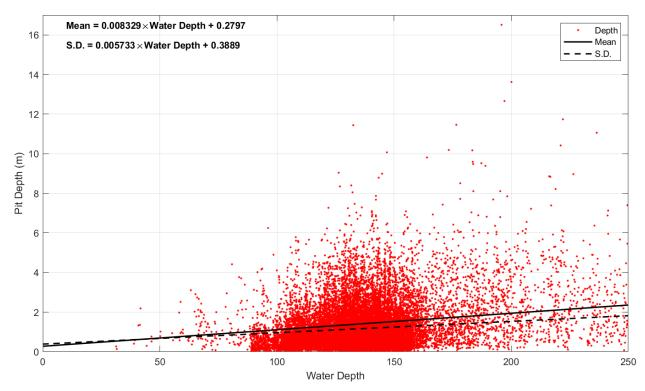
Figure 10. Pit depth as a function of water depth, Makkovik Bank region
