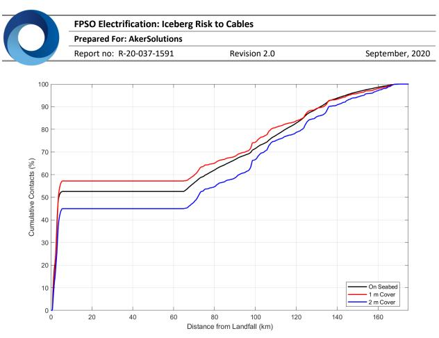
Figure 22. Cumulative iceberg contact risk for cable on seabed and trenched with 1 and 2 m cover
