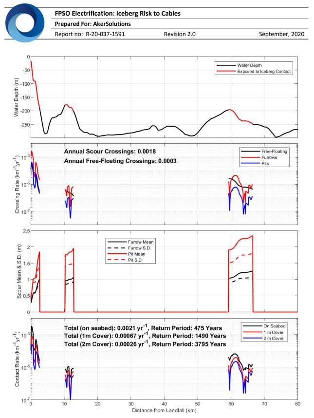
Figure 26. West Orphan Basin cable risk analysis (Trinity Bay landfall): portions of route exposed to icebergs, iceberg crossing rates over the cable, furrow and pit depth parameters, and contact rates
