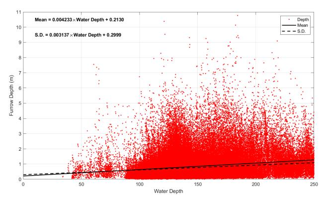
Figure 9. Furrow depth as a function of water depth, Makkovik Bank region
