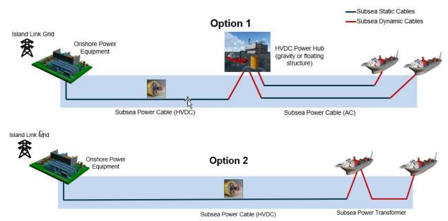
Figure 8-5: HVDC power from shore potential solutions
