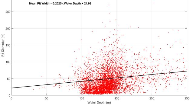
Figure 8. Mean pit diameter as a function of water depth, Makkovik Bank region
