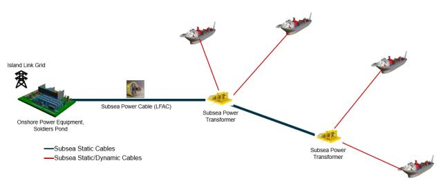
Figure 1-3: Representation of a LFAC power from shore transmission system for 4xFPSOs
