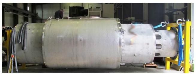
Figure -: BZ-25 MVES – Ex o, IP66, 9 × 35kV @ 400A sliprings, approximately 8.5m tall – Focal
