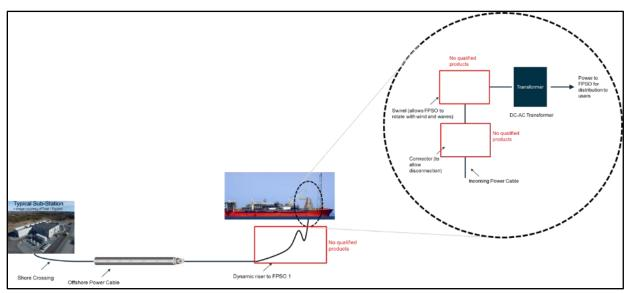
Figure 7-1: HVDC Power Supply to Ship Shaped FPSO
