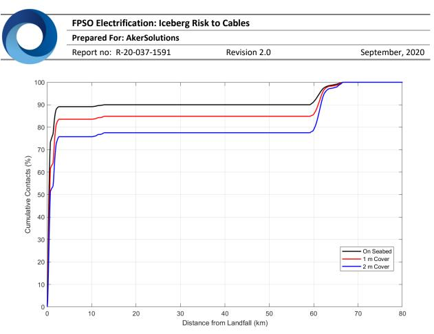
Figure 27. Cumulative iceberg contact risk for cable on seabed and trenched with 1 and 2 m cover
