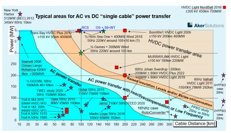
Figure 6-2: Subsea electrification project transmission technologies, loads, and distances
