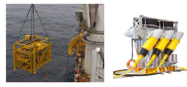
Figure 8-20: 19 MVA Aker Solutions Åsgard subsea compressor transformer module (left) and ABB subsea transformer unit (left) The Mecon 145kV Dry Mate connection is shown with yellow paint.
