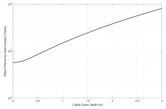
Figure 28. Mean return periods for cable contact as a function of cover depth
