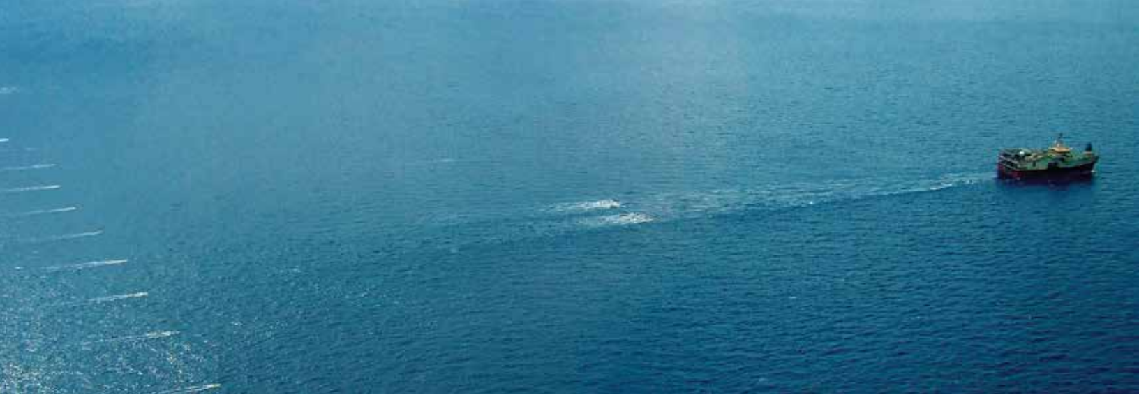
The hydrophone streamers deployed on a typical seismic survey can be up to one mile wide.
