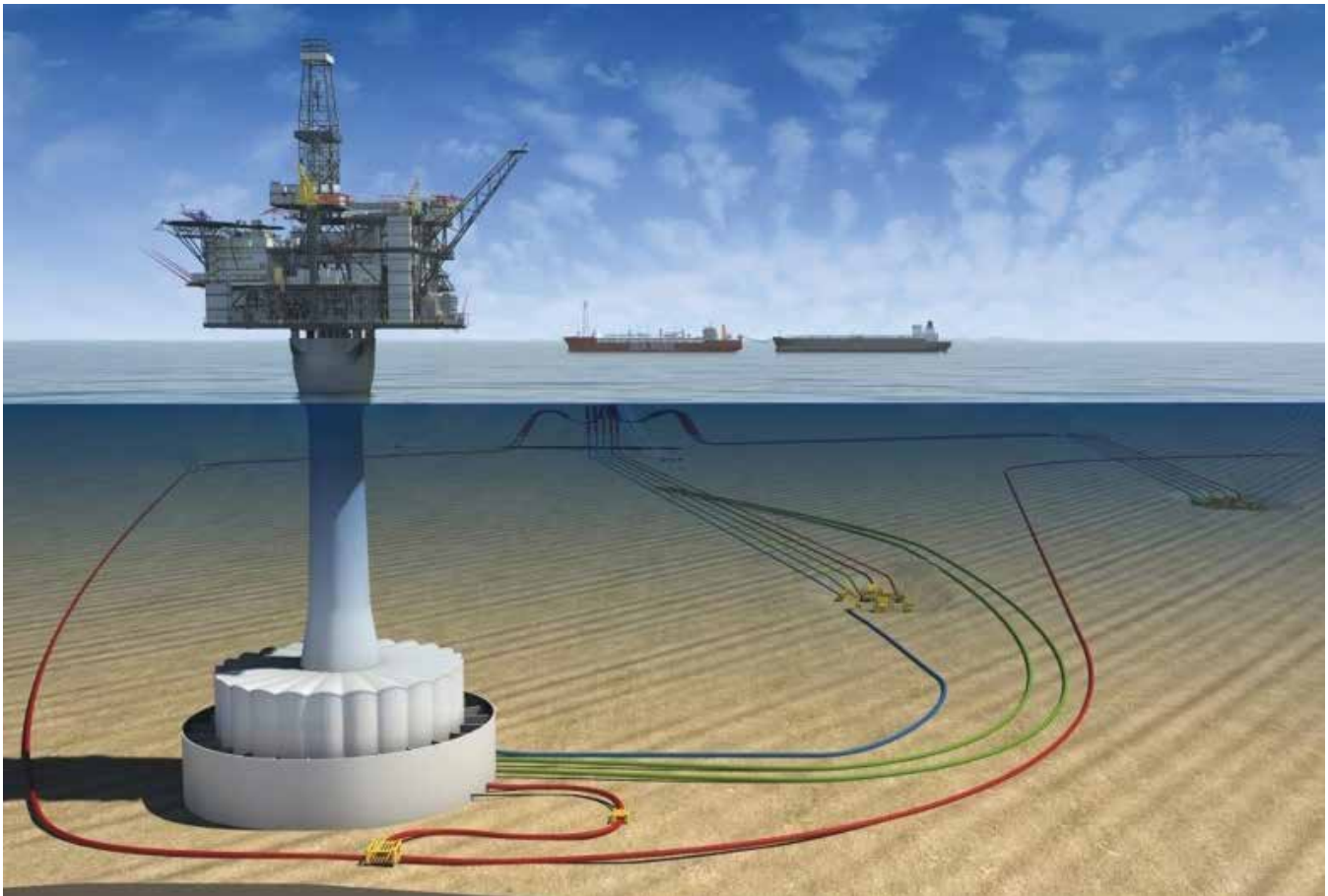
The West White Rose project will consist of a wellhead platform supported by a concrete base structure (CGS). Topsides components will include drilling facilities, wellhead and support services (accommodations, utilities, flare boom, helideck, lifeboat stations). Diagram courtesy of Husky Energy.
